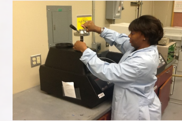
Step 2: Mount sample using bakelite molding. (Total time 22 min)
