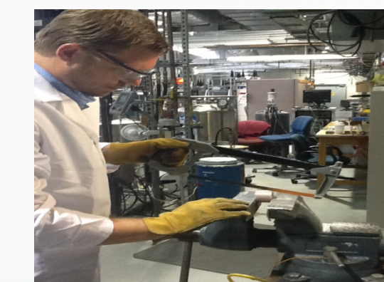
Step 1: Cut the Zylon based fiber samples from the winding.
