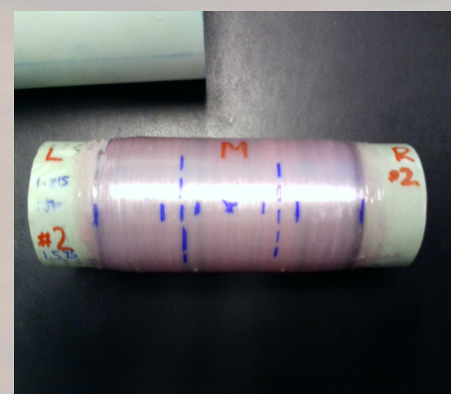
Zylon is wrapped around a winding which includes of glass fiber, Zylon fibers, and epoxy composite.
