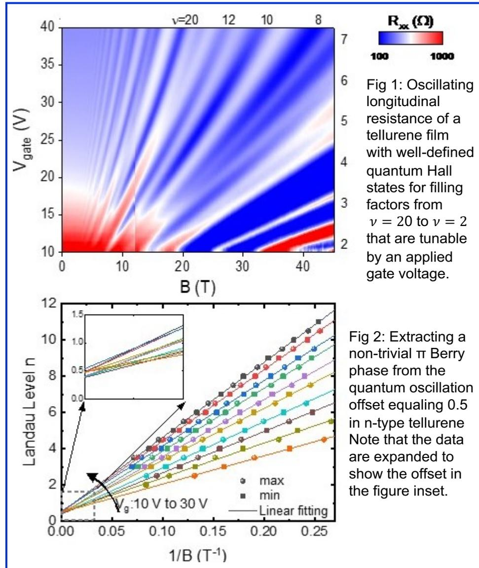
Fig 1: Oscillating longitudinal resistance of a tellurene film with well-defined quantum Hall states for filling factors from  $\nu = 20$  to  $\nu = 2$  that are tunable by an applied gate voltage.
