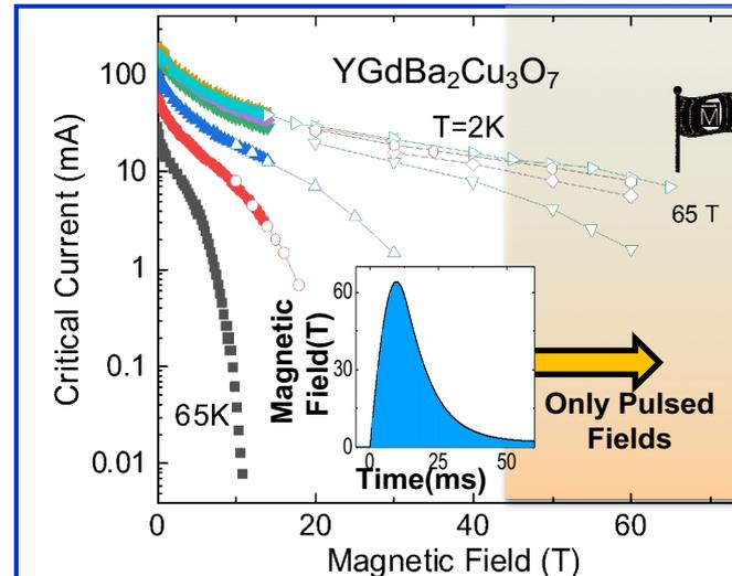
Measuring non-linear electric field – current density ( $E$ - $J$ ) curves in pulsed magnetic fields to 65T allowed researchers to determine critical current densities ( $J_c$ ) at record high magnetic fields.
