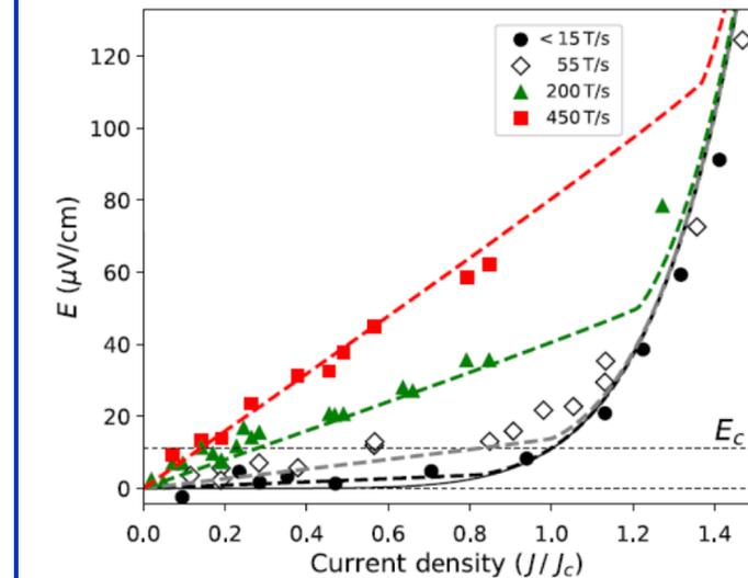
The data revealed new vortex physics from the  $E$ - $J$  curves measured in rapidly-changing magnetic fields. The collaboration developed a model that quantitatively describes the curves with no free parameters.
