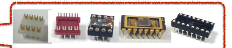
Various style of Dip header can be used as a sample holder **as long as** it meets the acceptable dimension above.
